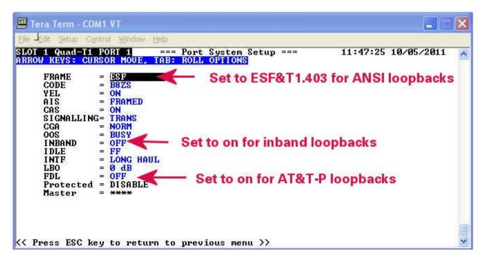
The following screen shows how to move around the screen and activate and deactivate loopbacks. The bottom of the screen shows if a command was successful or not.
