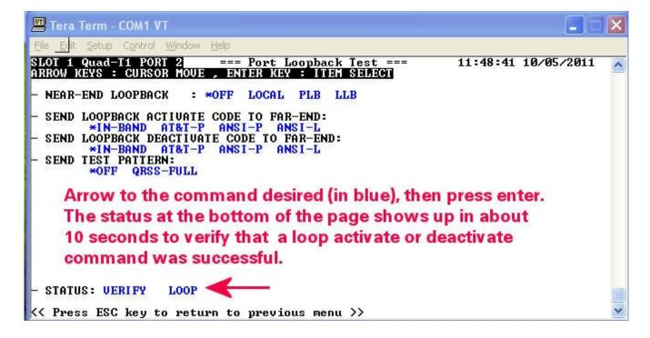
The T1 Port Loopback Test screen shows QRSS test results. When first turned on, the QRSS test may show a few bit errors. It is a 20 bit shift pattern that repeats every 1,048,575 bits.
